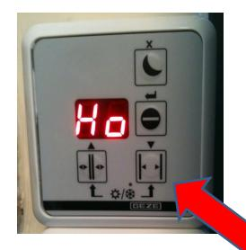
With door unlocked press the bottom right button. The key pad display will show 'Ho' (for Hold Open)
