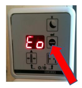
With door unlocked press the central right button. The key pad display will show 'Eo' (for Exit Only)
