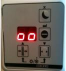
To **enable** the key pad turn the key a quarter turn clockwise. This is enable the key pad and the display will show two 'o's.
