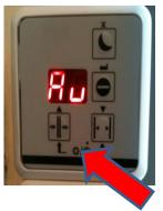
To operate the automatic door press the button on the bottom left of the key pad and the display will show 'Au' (for Automatic)
